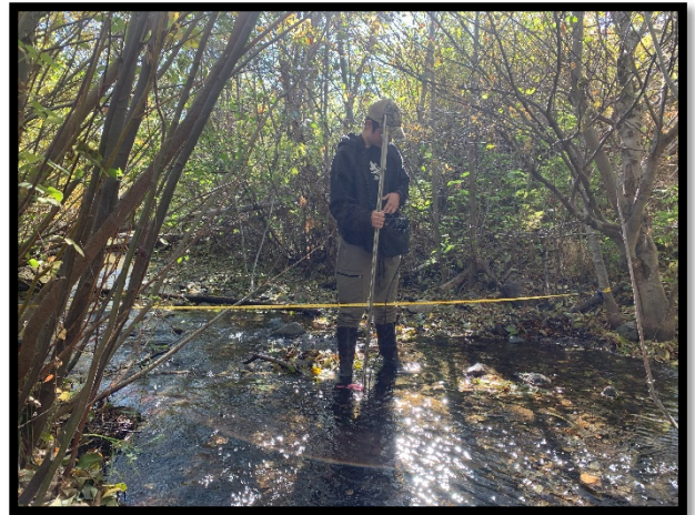
Figure 2. (Above): GrizzlyCorps Fellow, Clay Groetsch, assists with the final discharge measurements of the season for West Weaver Creek below the West Weaver Restoration Site.
